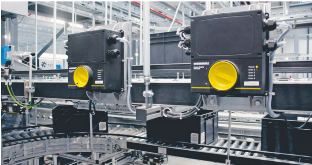
Efficient power supply: The robust, ready-to-use switched-mode power supplies with IP54 degree of protection are mounted directly where the protective extra-low voltage is needed, and not in the control cabinet. This allows much shorter cable lengths. The result is very short cables, which reduce power and material consumption and reduce faults such as a possible drop in line voltage, as well as a positive contribution to occupational safety.
