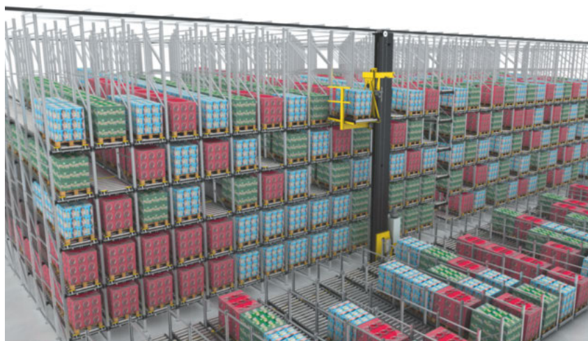
Stacker cranes and transfer cars as an extension of the MPP enable the continuous linking of automated conveying with automated warehouse processes.
