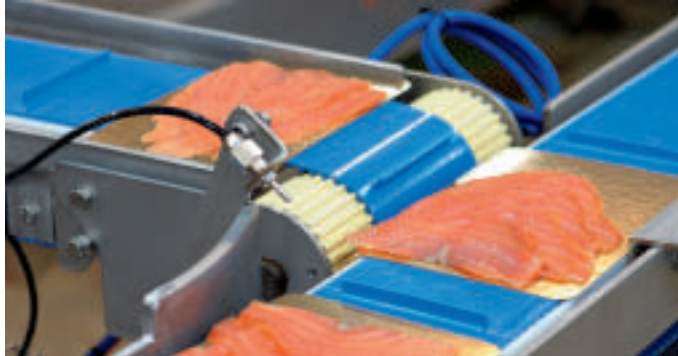
Ideal for high-frequency start-stop operation: new Synchronous Drum Motor as a conveyor belt drive for salmon processing
