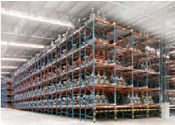
Motorcycles in space-saving dynamic stores: first in, first out – first-store pallets are first
