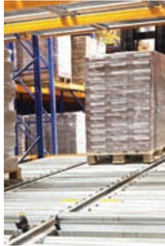
Gravity saves energy costs: Loading units "flow" on slightly inclined roller conveyors through the channels
