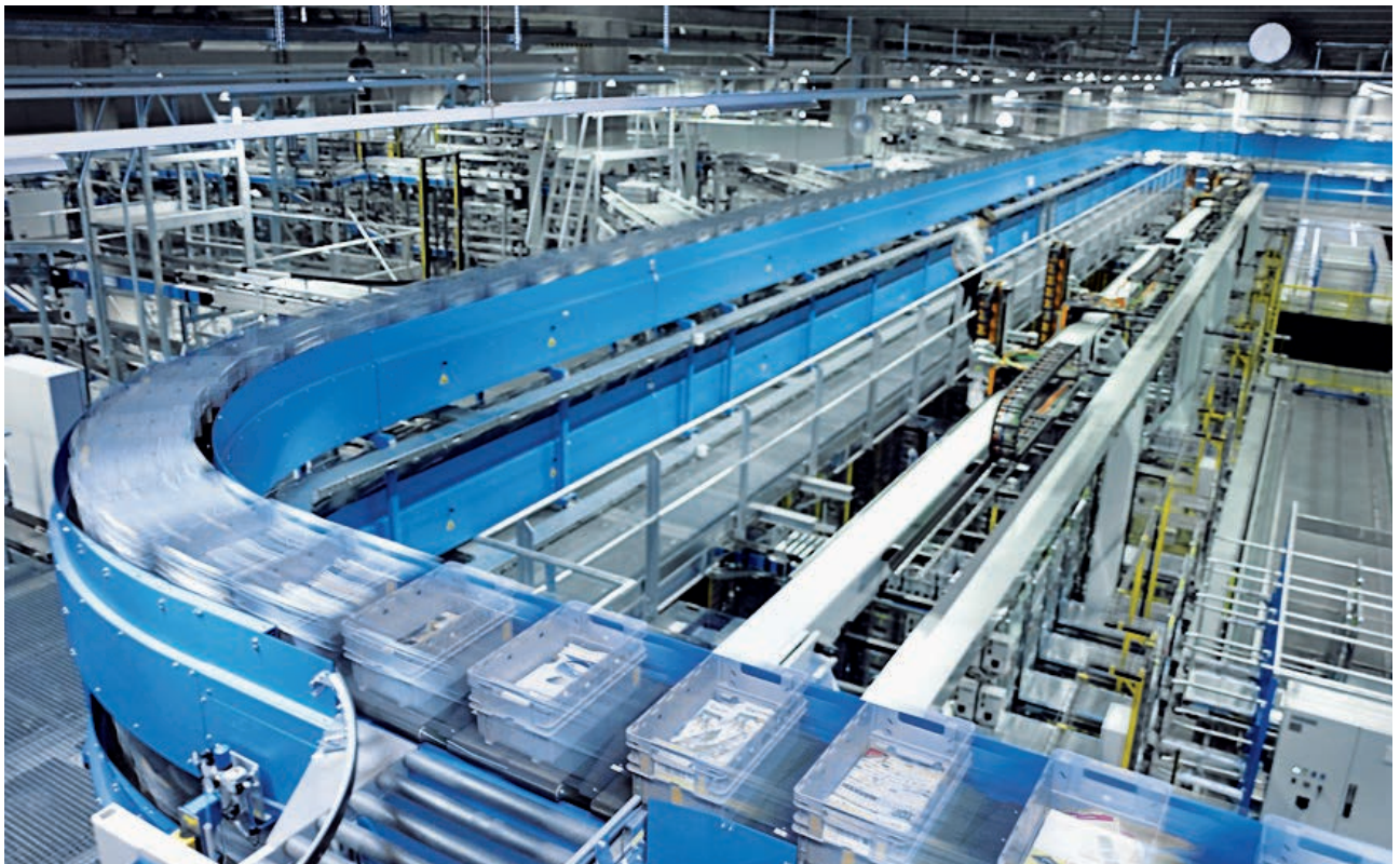
Interroll crossbelt sorters are installed at CEP (courier-express-parcel) providers all over the world.
