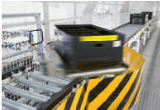
Intelligent, energy-saving conveyors: individual conveyor zones remain on stand-by until required.
