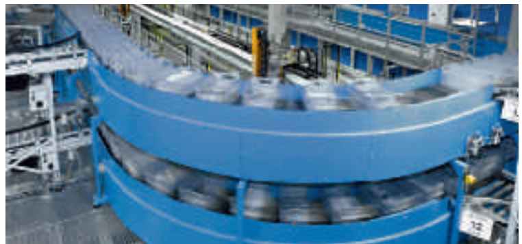
Interroll drum motors drive the conveyors at a poultry processing plant (left). Interroll crossbelt sorters carrying trays in the mail centre operated by Swiss Post in Zürich-Mülligen (right).
