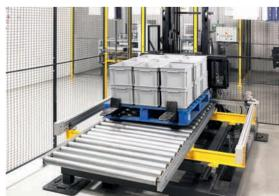
Repeated cycles to limit figures to determine the service life of the loading module
